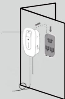
Lock the anti-theft screw on the top of the charging pile, and place the plug seat in an appropriate place
