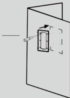
Install the charging pile on the backplane on the wall
