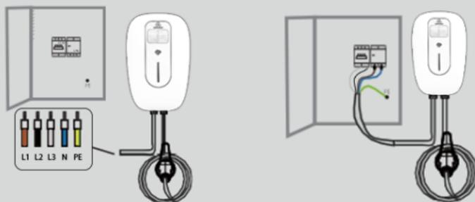
If the joint is connected, the heat shrinkable waterproof joint should be used to connect both ends. Notice that L1,L2,L3,N, PE correspond, Squeeze the joint with crimping pliers to ensure good contact
